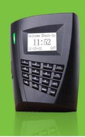
SC503 is an access control device produced by which is made with elegant design and professional surface treatment. The device has lock control, alarm, exit button and door sensor. The wiegand-in interface is used to connect external reader to construct master and slave system. Also, the device can be used to connect with a control panel as a reader by wiegand-out interface.
